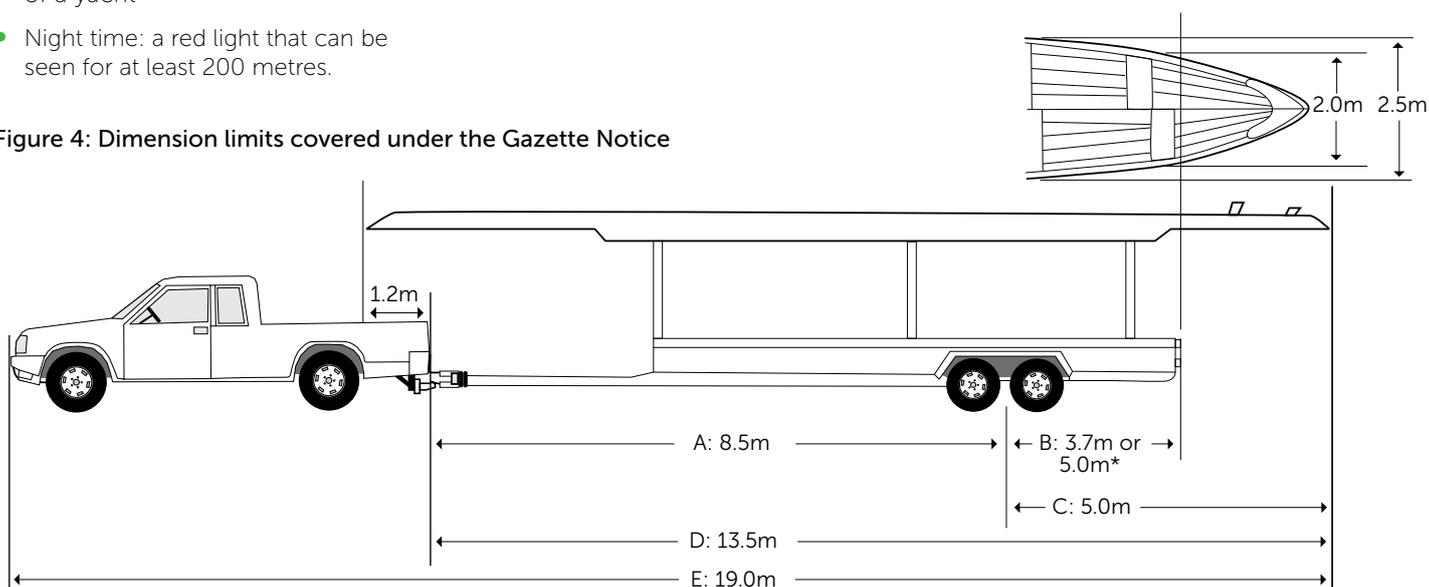
\*The rear overhang of a glider trailer as constructed must not exceed 5.0m
